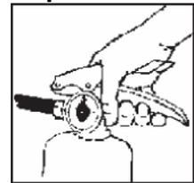
Squeeze the lever on the fire extinguisher.
